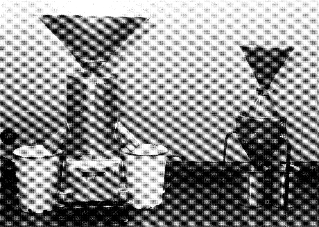
Figure 15.3. Subsampling dividers: on the left is a Gamet Precision divider and on the right is a Boerner divider (Courtesy of Bob Neumann).
