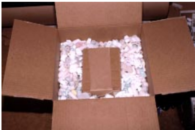
Fig. 34. A box of specimens being readied for shipment. Note that ample room has been left on all sides of the specimen container for cushioning material.
