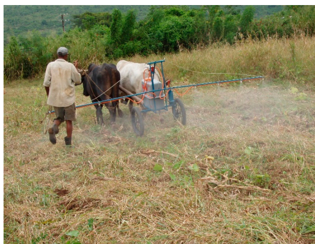
Figure 5. An animal-drawn sprayer for weed and cover crop management. The 80-L tank supplies a 5 m spray boom via a ground-wheel driven pump (Photo: B Sims).
