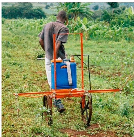
Figure 4. A knapsack sprayer fitted to a wheeled chassis. The four nozzles give a uniform 2 m-wide spray swath well to the rear of the operator (Photo: B Sims).
