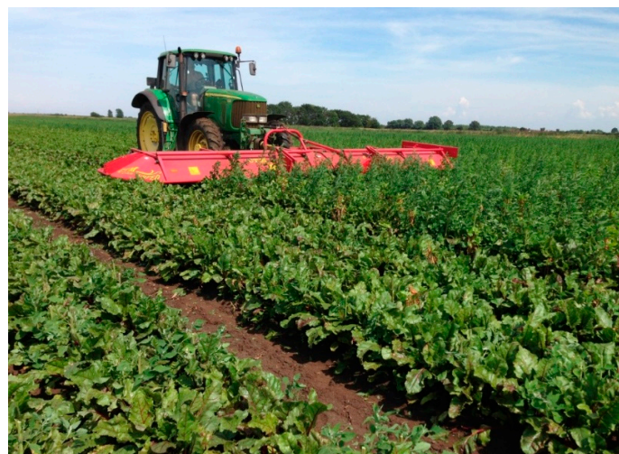
Figure 3. A weed header (Weed Surfer) in action topping weed seed heads protruding above an organic beetroot ( Beta vulgaris L.) crop (Photo: S Briggs).
