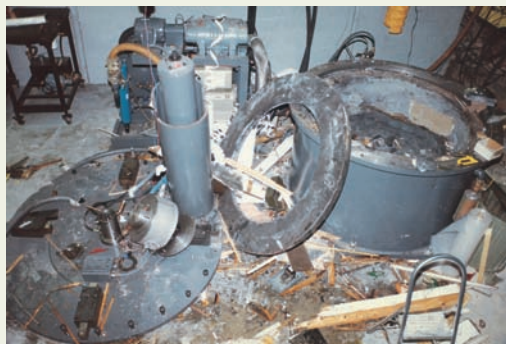
Fig. 10-15 Some of the destruction caused by the explosion of a rapidly rotating steel disk. (Courtesy Test Devices, Inc.)
