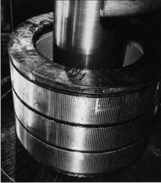
FIGURE 7-19 A closeup of the commutator of a large lap-wound dc machine. The equalizers are mounted in the small ring just in front of the commutator segments. (Courtesy of General Electric Company.)
