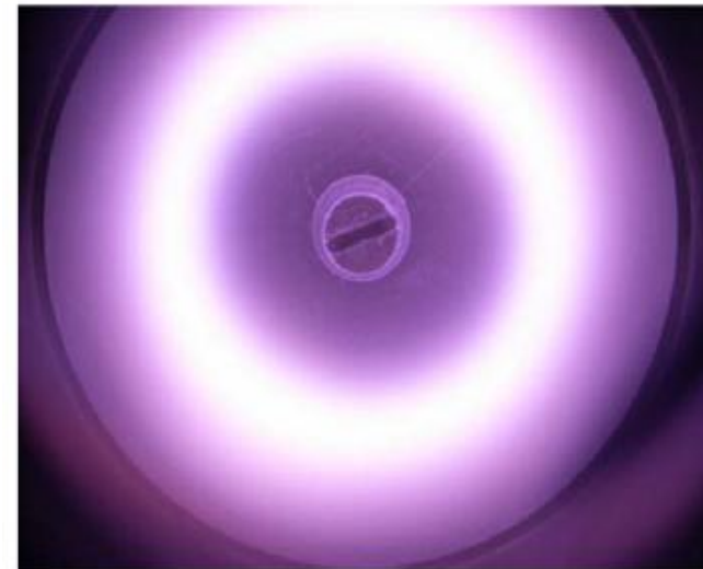
Figure 5.9: Simulated part of a trajectory of an electron on a circular planar magnetron (a) and the resulting torus-shaped argon plasma (b).
