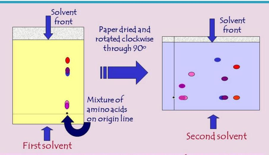
Two-way chromatography provides better separation of substances that behave in a similar fashion in the first solvent. A second run in a different solvent resolves two very close spots more clearly
