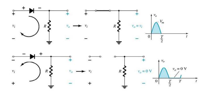
The DC output voltage is  $0.318V_m$ , where  $V_m$  = the peak AC voltage.
