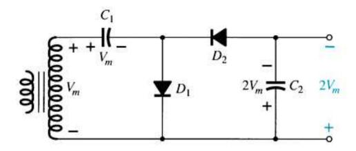
This half-wave voltage doubler's output can be calculated by:
