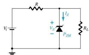
If R is too small, the Zener current exceeds the maximum current rating,  $I_{ZM}$ . The maximum current for the circuit is given by:
