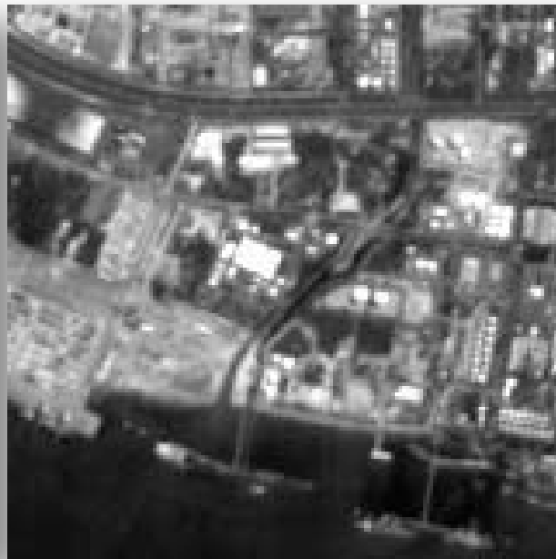
6-bit quantization (64 levels)
