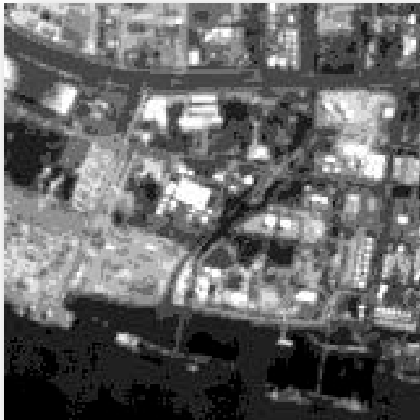
3-bit quantization (8 levels)
