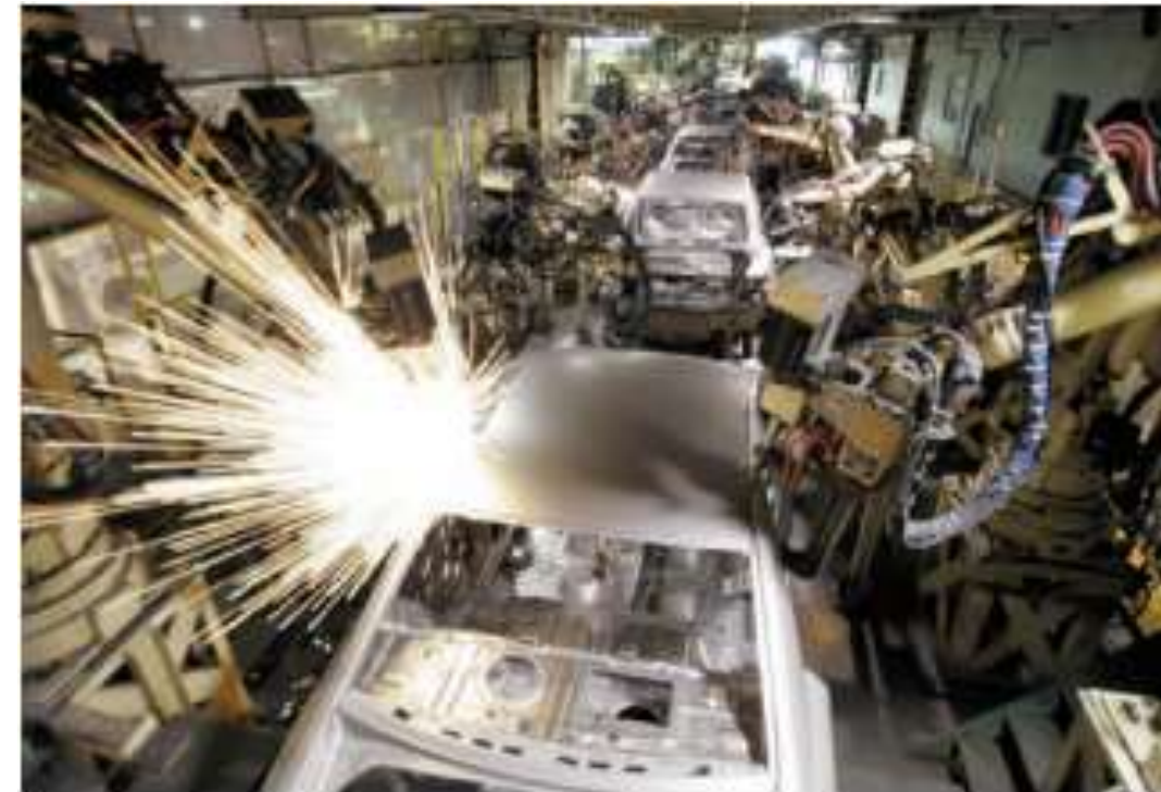
Figure 1-38 Automotive factories use industrial robots to weld car bodies.
