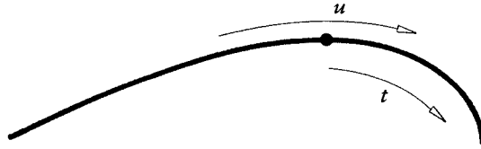
Figure 11.9 G^r continuity: a segment of a C^r curve may be reparametrized. The resulting curve is not C^r anymore, but still G^r .
