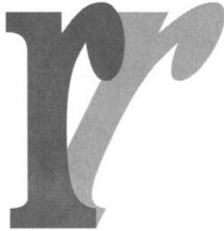
Figure 2.4 A shear: this affine map is used in font design in order to generate slanted fonts. Dark gray: original letter; light gray: slanted (sheared) letter.
