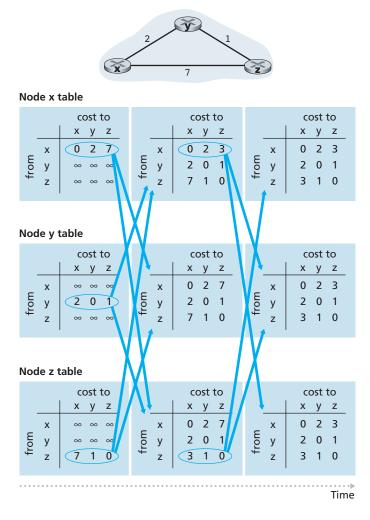
Figure 4.30 ♦ Distance-vector (DV) algorithm
