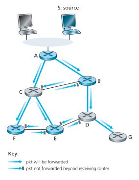
Figure 4.50 ♦ Reverse path forwarding, the multicast case
