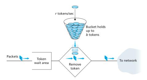
Figure 7.23 ◆ The leaky bucket policer
