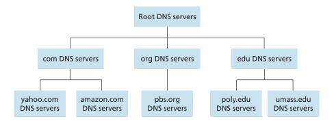
Figure 2.19 ♦ Portion of the hierarchy of DNS servers
