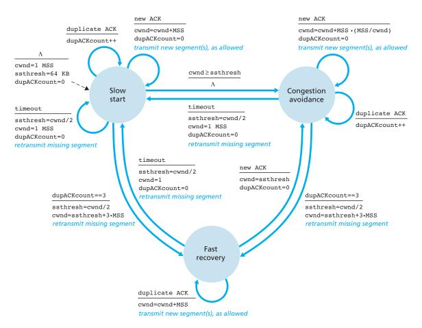
Figure 3.52 ◆ FSM description of TCP congestion control
