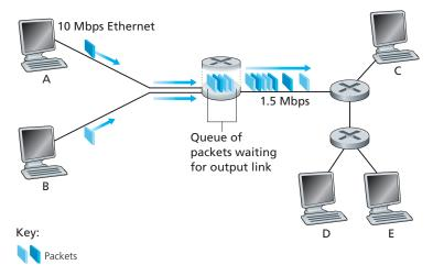
Figure 1.12 ◆ Packet switching
