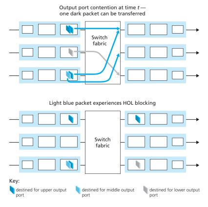
Figure 4.11 ♦ HOL blocking at an input queued switch
