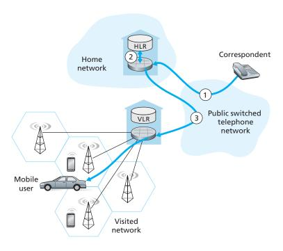
Figure 6.29 ♦ Placing a call to a mobile user: indirect routing
