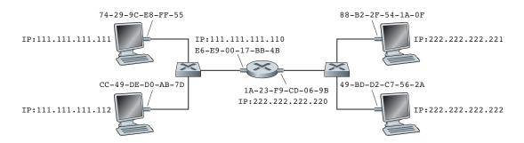
Figure 5.19 ♦ Two subnets interconnected by a router
