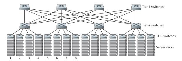
Figure 5.31 ♦ Highly-interconnected data network topology
