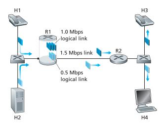
Figure 7.16 ♦ Logical isolation of audio and HTTP traffic classes
