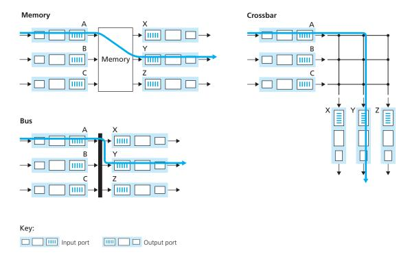
Figure 4.8 ♦ Three switching techniques
