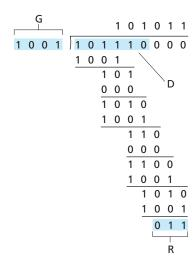
Figure 5.7 ♦ A sample CRC calculation
