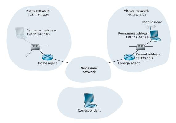
Figure 6.22 ♦ Initial elements of a mobile network architecture
