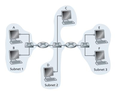
Figure 5.33 ◆ Three subnets, interconnected by routers
