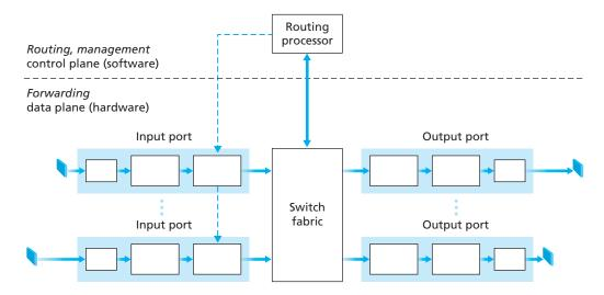
Figure 4.6 ♦ Router architecture
