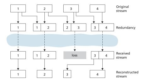
Figure 7.8 ♦ Piggybacking lower-quality redundant information
