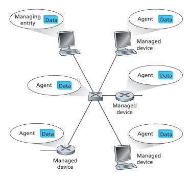
Figure 9.2 ♦ Principal components of a network management architecture
