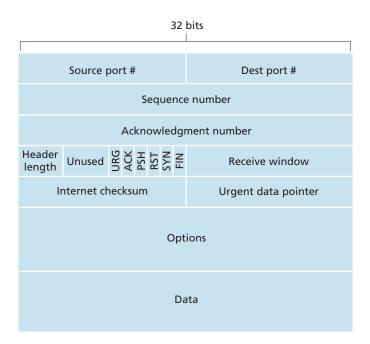
Figure 3.29 ♦ TCP segment structure
