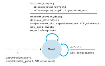
Figure 3.21 ♦ Extended FSM description of GBN receiver
