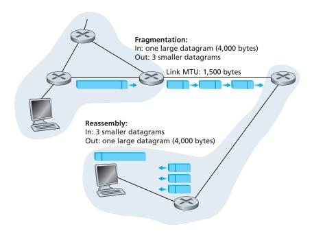
Figure 4.14 ♦ IP fragmentation and reassembly
