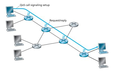
Figure 7.28 ♦ The call setup process
