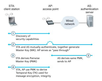
Figure 8.31 ♦ 802.11i: four phases of operation
