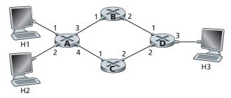
P5. Consider a VC network with a 2-bit field for the VC number. Suppose that the network wants to set up a virtual circuit over four links: link A, link B,
