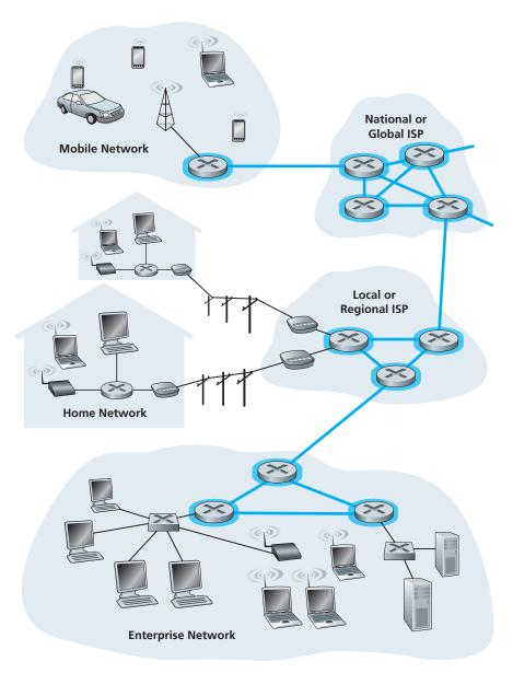
Figure 1.10 ♦ The network core
