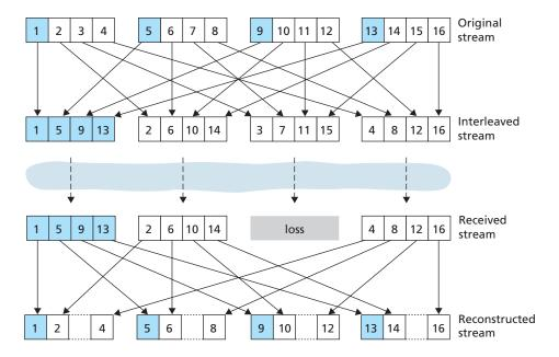
Figure 7.9 ◆ Sending interleaved audio
