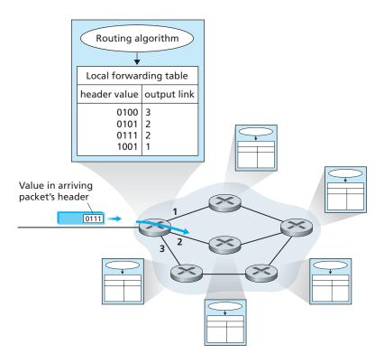
Figure 4.2 ◆ Routing algorithms determine values in forwarding tables
