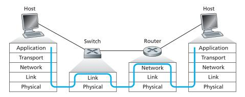
Figure 5.24 ♦ Packet processing in switches, routers, and hosts
