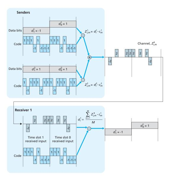
Figure 6.6 ♦ A two-sender CDMA example
