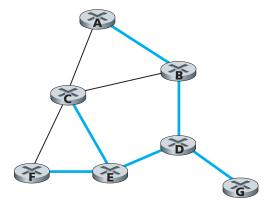
b. Constructed spanning tree
