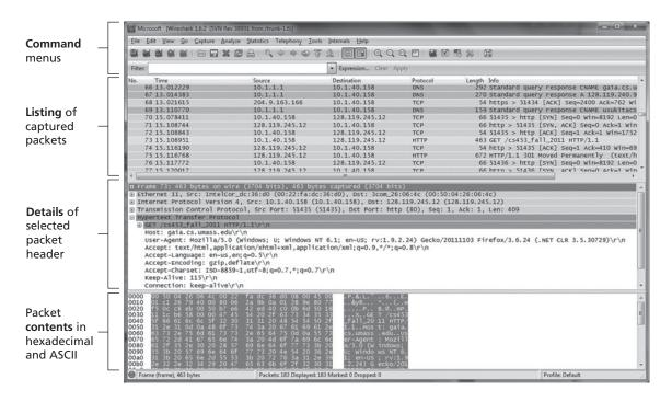
Figure 1.28 • A Wireshark screen shot (Wireshark screenshot reprinted by permission of the Wireshark Foundation.)
