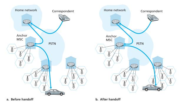
Figure 6.32 ♦ Rerouting via the anchor MSC
