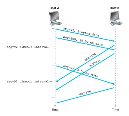
Figure 3.35 ◆ Segment 100 not retransmitted
