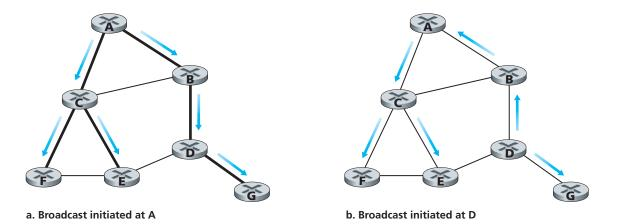
Figure 4.45 ♦ Broadcast along a spanning tree
