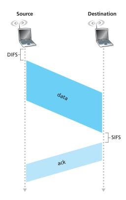
Figure 6.10 ♦ 802.11 uses link-layer acknowledgments
