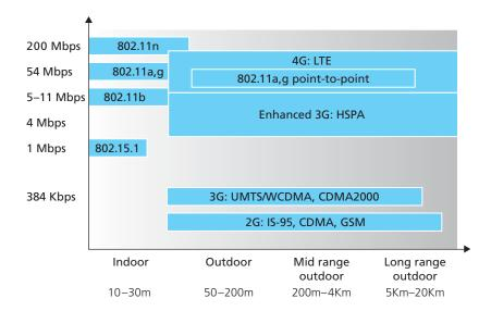
Figure 6.2 ♦ Link characteristics of selected wireless network standards
