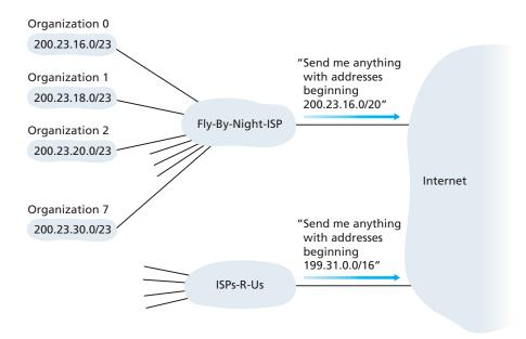
Figure 4.18 ♦ Hierarchical addressing and route aggregation
