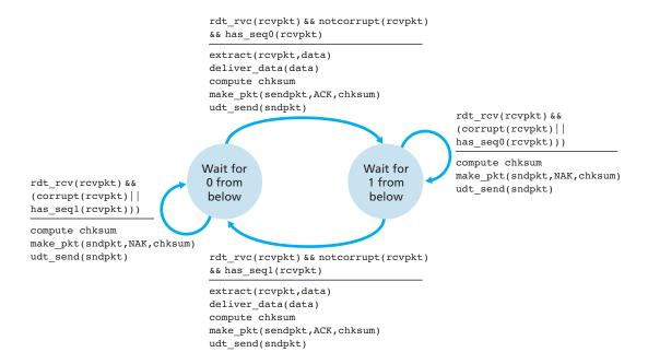
Figure 3.57 ♦ An incorrect receiver for protocol rdt 2.1
