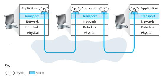
Figure 3.2 ♦ Transport-layer multiplexing and demultiplexing
