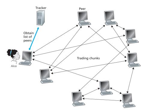
Figure 2.26 ♦ File distribution with BitTorrent
