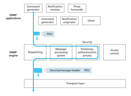
Figure 9.5 ◆ SNMPv3 engine and applications
