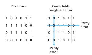
Figure 5.5 ♦ Two-dimensional even parity
