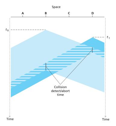
Figure 5.13 ◆ CSMA with collision detection
