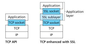
Figure 8.24 ♦ Although SSL technically resides in the application layer, from the developer's perspective it is a transport-layer protocol
