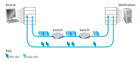
Figure 3.50 ♦ Congestion-control framework for ATM ABR service
