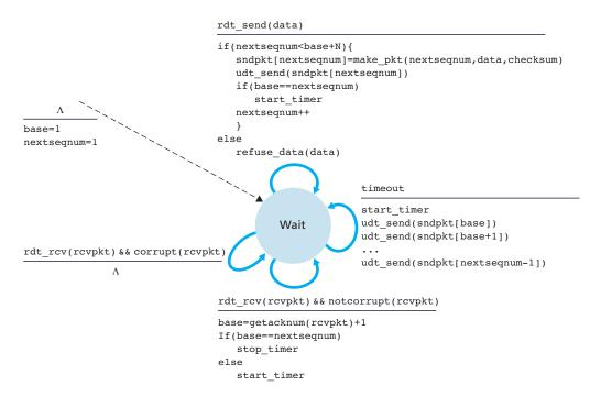
Figure 3.20 ♦ Extended FSM description of GBN sender
