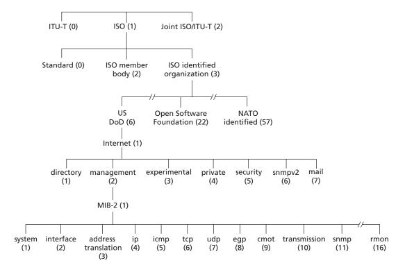
Figure 9.3 ♦ ASN.1 object identifier tree
