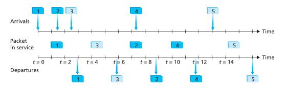
Figure 7.21 ◆ Operation of the two-class round robin queue
