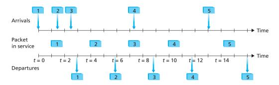
Figure 7.18 ◆ The FIFO queue in operation
