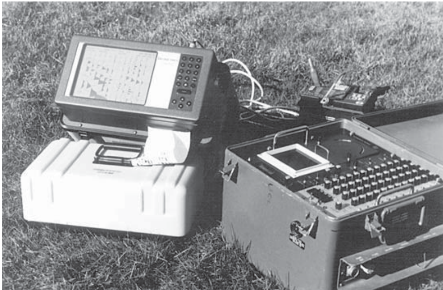
Figure 11.9 Enhancement seismographs. The instrument on the right is the now obsolete knob and switch controlled Geometrics 1210F. The instrument on the left is one of its successors, the Smartseis, which is entirely menu-driven. Note the hard-copy record just emerging from the Smartseis, and the much greater size of the display 'window'.
