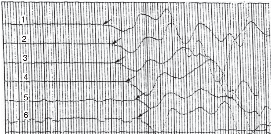
Figure 11.10 Six-channel refraction record showing refraction ‘picks’. Noise prior to these picks is increasingly obvious as amplification is increased to record signals from the further geophones.
