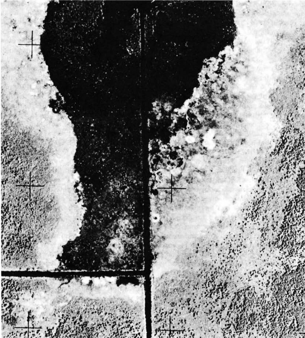
Figure 4.32 Black and white copy of a color infrared aerial photograph of Sheboygan Marsh, WI. Scale 1:9000 (enlarged 6.7 times from 1:60,000). Grid ticks appearing in image are from a reseau grid included in camera focal plane. (NASA image.)
