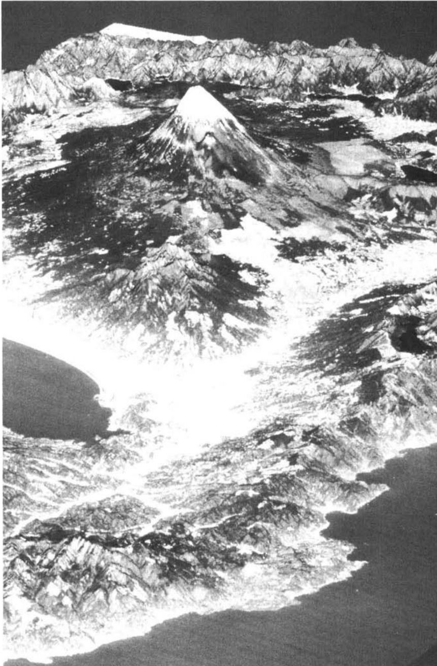
Figure 7.59 Perspective-view image of Mount Fuji, Japan, produced by combining Landsat TM data (bands 2, 3, and 4, shown in black and white) and digital elevation model (DEM) data. (Copyright © RESTEC/NIHON University, 1991.) (Figure 8.45 shows a radar image of this area as well.)
