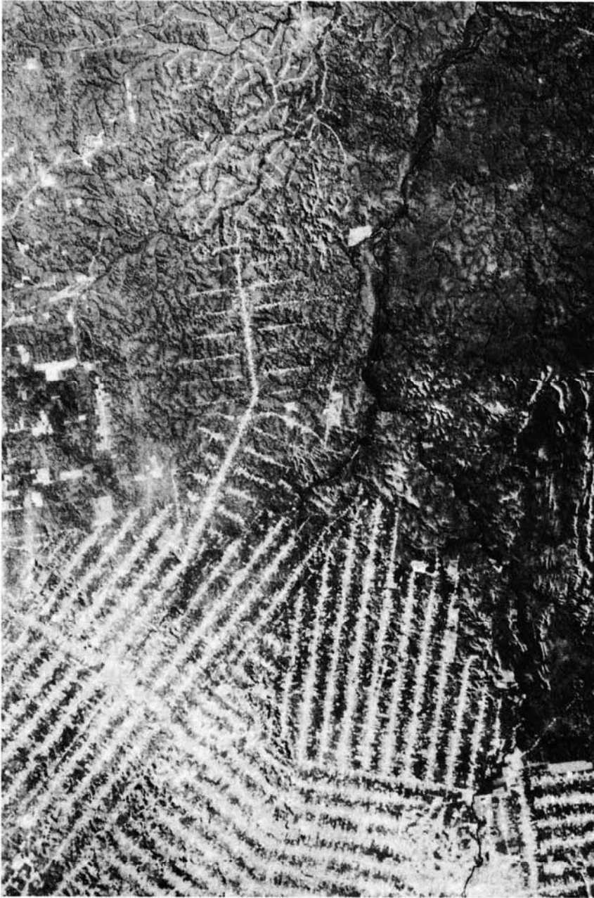
Figure 6.20 Landsat TM image, Rondônia, Brazil, and vicinity, mid-August. Black and white copy of band 3–4–5 color composite image. Scale 1:1,000,000. (Courtesy EOSAT.)
