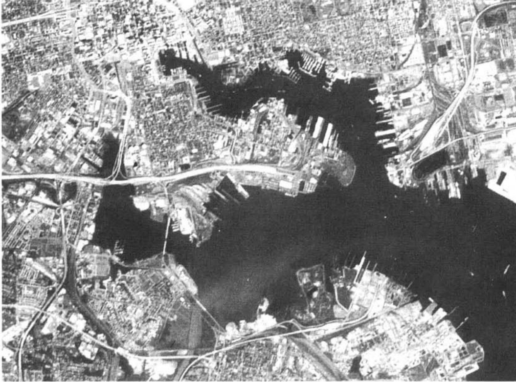
Figure 6.26 SPOT-1 panchromatic image, Baltimore, MD, Inner Harbor, late August. Scale 1:70,000. (Copyright © 1986 CNES. Courtesy SPOT Image Corp.)
