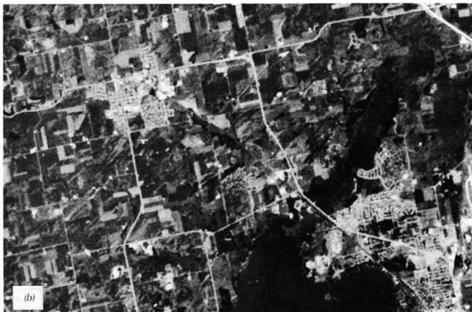
Figure 6.17 Individual Landsat TM bands, suburban Madison, WI, late August (scale 1:115,000): (a) band 1, 0.45 to 0.52 \mu\text{m} (blue); (b) band 2, 0.52 to 0.60 \mu\text{m} (green); (c) band 3, 0.63 to 0.69 \mu\text{m} (red); (d) band 4, 0.76 to 0.90 \mu\text{m} (near IR); (e) band 5, 1.55 to 1.75 \mu\text{m} (mid IR); (f) band 7, 2.08 to 2.35 \mu\text{m} (mid IR); (g) band 6, 10.4 to 12.5 \mu\text{m} (thermal IR).
