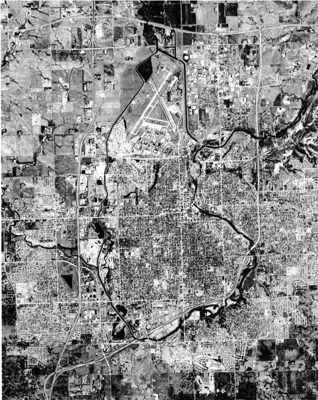
Figure 6.16 The first image acquired by the Landsat-7 ETM+. Panchromatic band (15 m resolution), Sioux Falls, SD, April 18, 1999. Scale 1: 88,000. (Courtesy EROS Data Center.)
