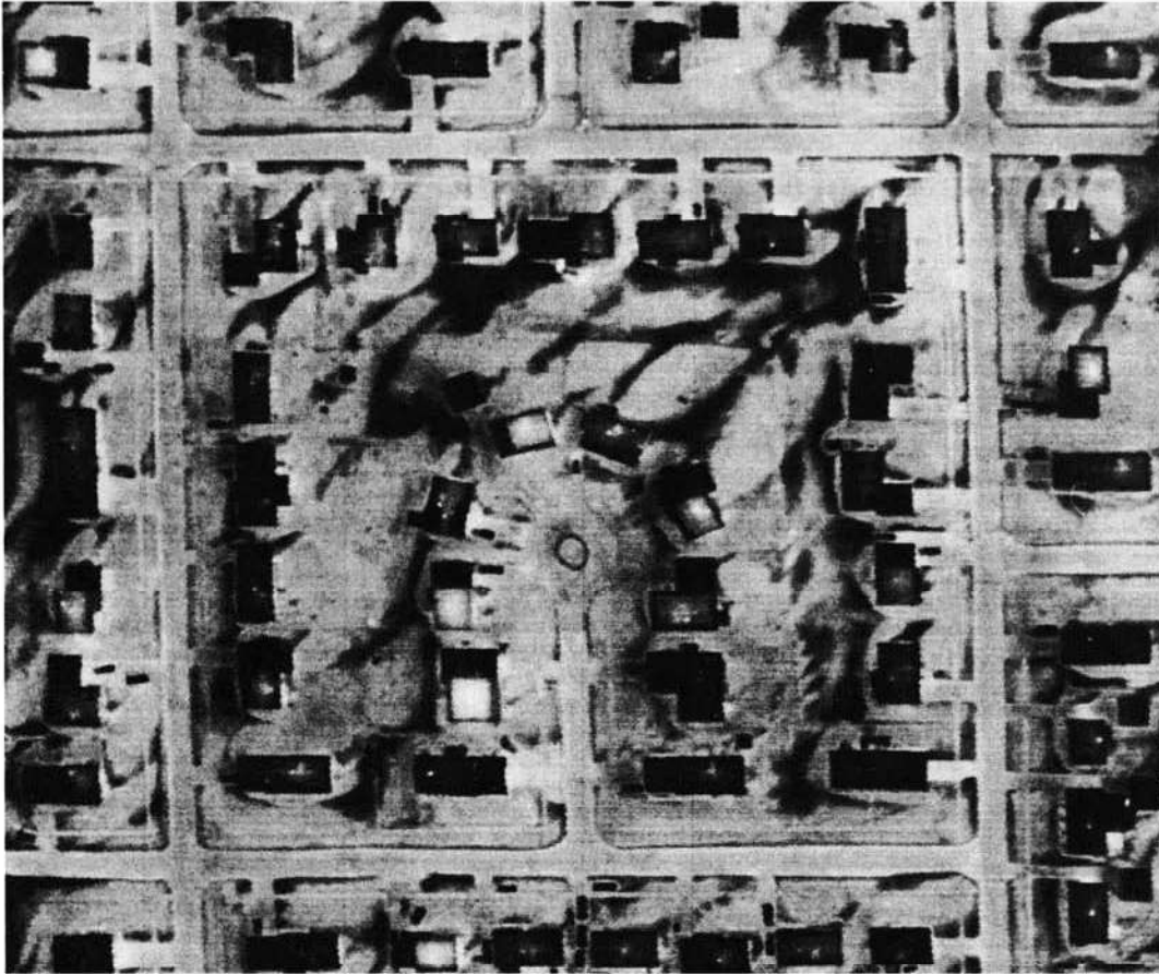
Figure 5.22 Nighttime thermal image depicting building heat loss in an Iowa City, approximately 2:00 A.M., snow-covered ground, air temperature approximately -4^{\circ}\text{C} , 460 m flying height, 1 mrad IFOV. (Courtesy Iowa Utility Association.)
