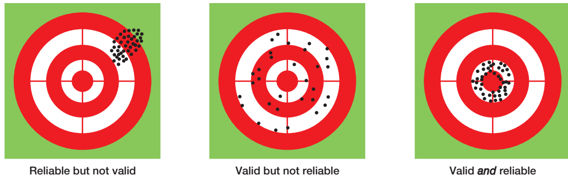
FIGURE 5-2 An Analogy to Validity and Reliability. A good measurement technique should be both valid (measuring what it is intended to measure) and reliable (yielding a given measurement dependably).
