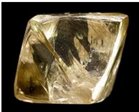
Figure 4a: The internal structure of diamond shows equally strong bonds in all directions. An uncut diamond crystal
