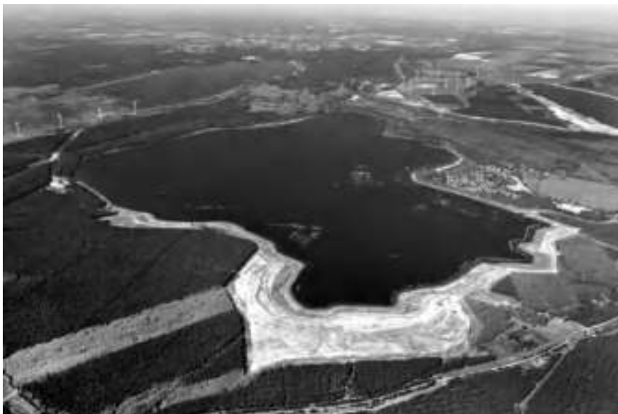
Figure 6.30 (Plate 6.30) Post-mining lignite open pit lakes in the Lausitz region, Germany, in the last stages of filling and rehabilitation. Courtesy of P. Radke, © LMBV, Lausitzer und Mitteldeutsche Bergbau-Verwaltungsgesellschaft mbH.
