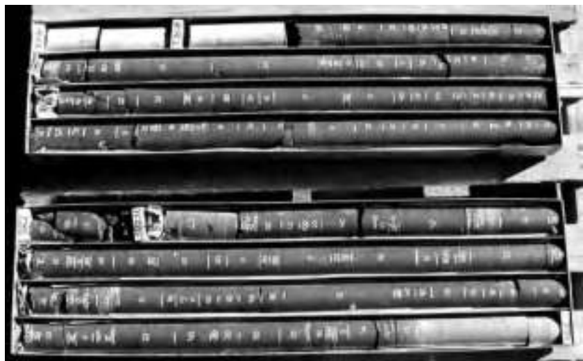
Figure 6.25 Slimline (HQ) drill core section of Permian Wallarah-Great Northern coal seam in the Sydney basin, New South Wales, Australia. Courtesy of Keith Bartlett, Minarco-Mineconsult, Tuggerah, NSW. Light shales in the footwall (foreground right) grade into bedded coal which is overlain by matrix-supported roof conglomerate (back, left). Figures marked in white on core denote brightness.
