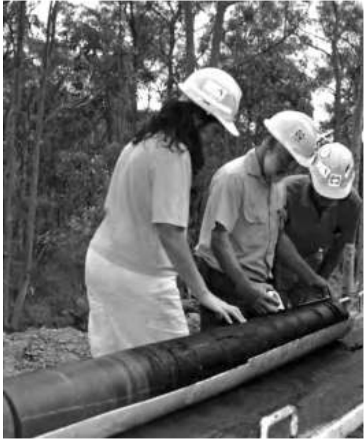
Figure 6.26 Large diameter core (200 mm diameter) is drilled for quantifying technological parameters of coal such as fragmentation and washability. Courtesy of Keith Bartlett, Minarco-Mineconsult, Tuggerah, NSW.
