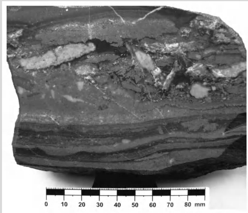
Figure 1.76 (Plate 1.76) Banded and breccia cave ore of brown sphalerite in the historic Lafatsch mine, Karwendel, Tyrol. This is one of the outliers of the Triassic Alpine type carbonate-hosted Pb-Zn deposits. Courtesy B. Lehmann, Clausthal.
