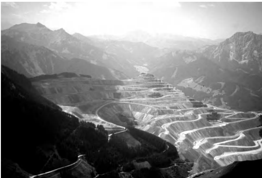
Figure 1.35 The metasomatic siderite deposit Erzberg (“ore mountain” in German) in Austria. The active quarry faces away from the camera. The view shows disposal of barren carbonate host rock.
