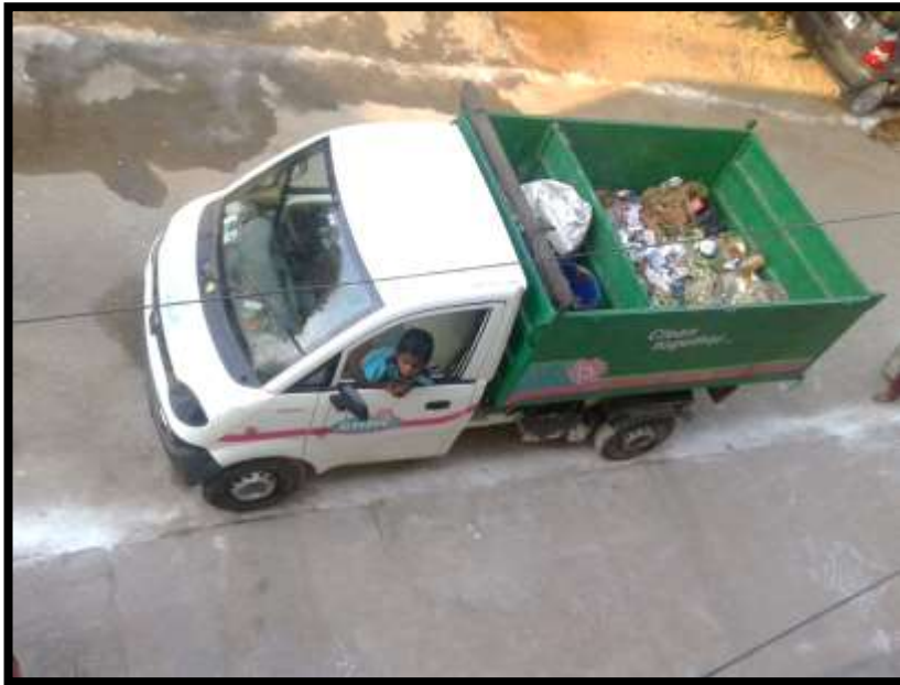
Figure 10 Separate slots for organic and recyclable waste in GHMC's door-to-door collection vehicle
