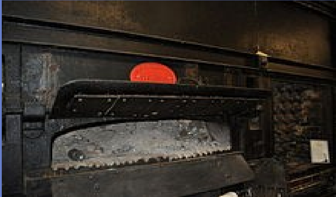
Manlove, Alliott & Co. Ltd. 1894 destructor furnace. The use of incinerators for waste disposal became popular in the late
