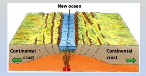
Magma solidifies to form *new crust* in the rift valley floor. Crustal blocks on either side slip down along a succession of steep faults, creating mountains. A narrow ocean is formed , floored by new oceanic crust.
