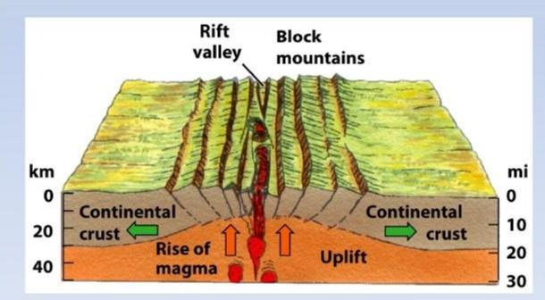
Crust is uplifted and stretched apart, causing it to break into blocks that become tilted on faults. Eventually long narrow *rift valley* appears. Magma rises up from the mantle to fill the widening crack at the center.
