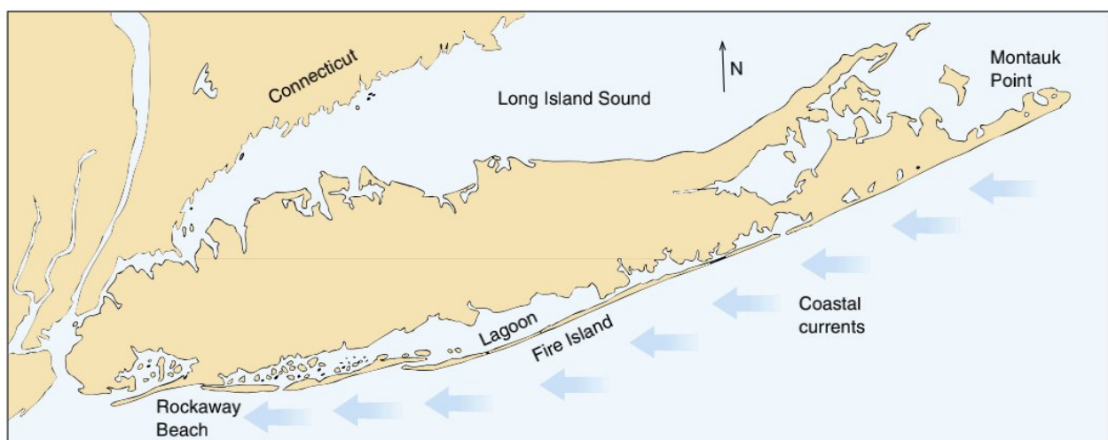
Figure 18–20 Longshore currents carry sand westward along the south shore of Long Island.
