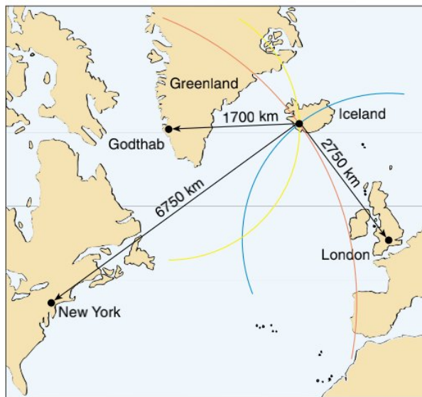
Figure 10-14 Locating an earthquake. The distance from each of three seismic stations to the earthquake is determined from time-travel curves. The three arcs are drawn. They intersect at only one point, which is the epicenter of the earthquake.
