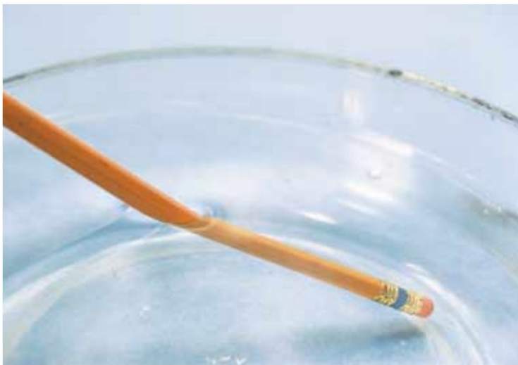
Figure 10–28 If you place a pencil in water, the pencil appears bent. It actually remains straight, but our eyes are fooled because light rays bend, or refract, as they cross the boundary between air and water.
