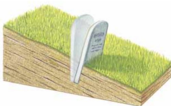
Figure 13-7 During creep, the soil surface moves more rapidly than deeper layers, so the tombstone embedded in the soil tilts downhill.
