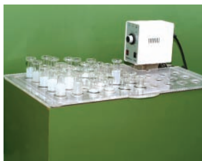
Figure 31. Circulating water bath with holder for syringes
