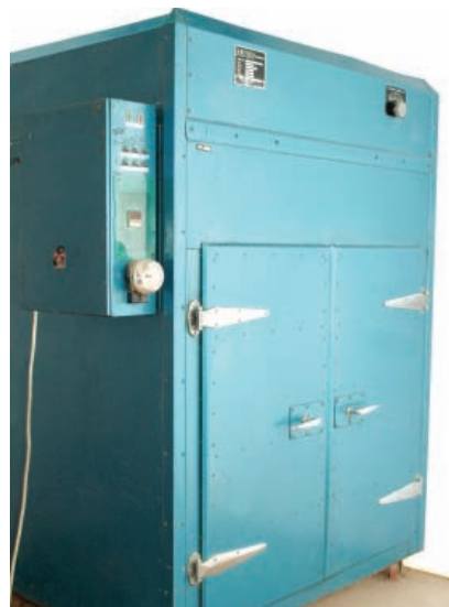
Figure 3. Air-circulation oven for field samples
