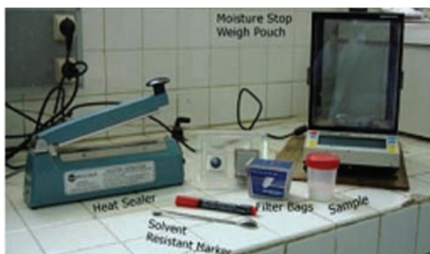
Figure 19. ANKOM bags, sealer, balance
