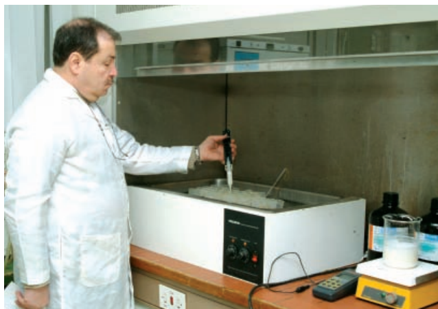
Figure 38. Water bath with centrifuge tubes, adding pepsin
