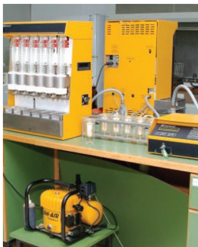
Figure 13. Soxhlet apparatus with control unit
