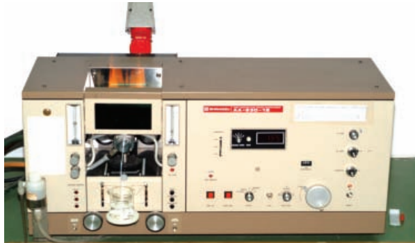
Figure 21. Atomic absorption and flame emission spectrophotometer
