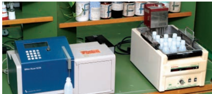
Figure 48. Milkoscan with water bath
