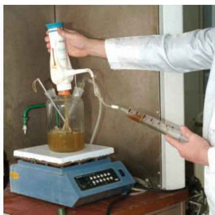
Figure 32. Heating plate with stirrer, Wouff bottle, and dispenser
