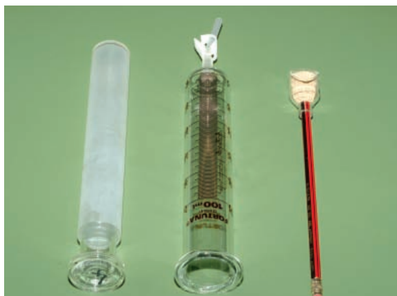
Figure 34. Syringe for GPT & weighing spatula
