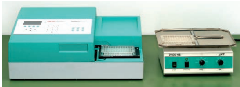
Figure 59. ELISA reader and plate shaker
