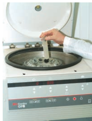
Figure 37. Centrifuge with centrifuge tubes
