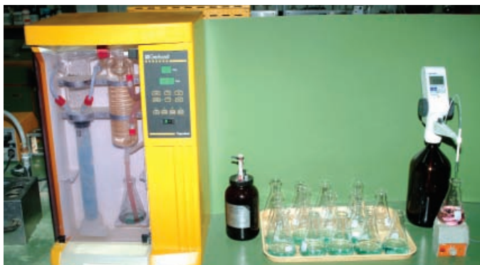
Figure 10. Automatic distillation unit (Kjeldahl) and automatic burette for titration
