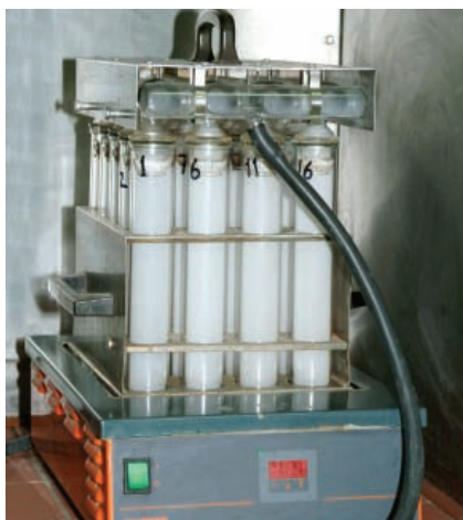
Figure 11. Digestion block heater with exhaust manifold
