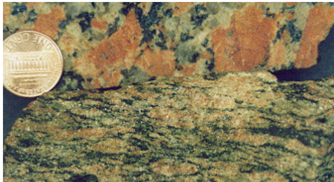
Figure 27. Granite (above) and gneiss (below) are composed of similar minerals. Note the irregular horizontal foliation in the gneiss defined by light and dark minerals.
