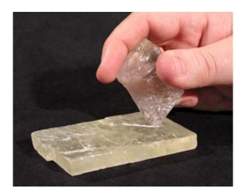
**Figure 4:** Testing mineral hardness. The harder mineral (quartz) scratches the softer one (calcite).
