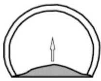
Heave of invert
