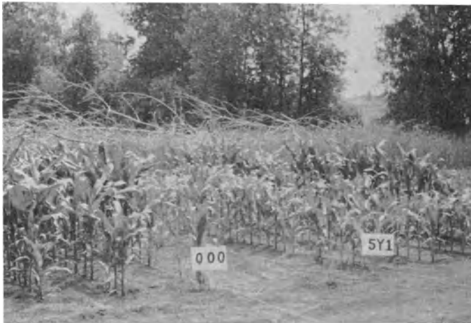
Figure 4. Left: corn on uncompacted (000) plots. Right: corn on plots subjected to 5 passes at contact pressure of 41 kPa (30 days after seeding).
