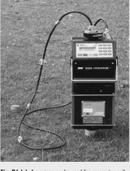
Fig. B6.1.1 A neutron probe used for measuring soil water content *in situ*.
