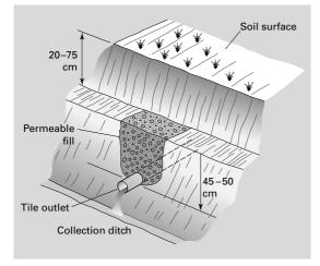
Fig. 13.12 Diagram of a tile drain imbedded in permeable fill.
