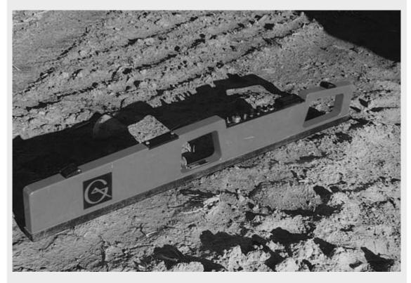
Fig. B13.3.1 An example of a portable EM38 meter.
