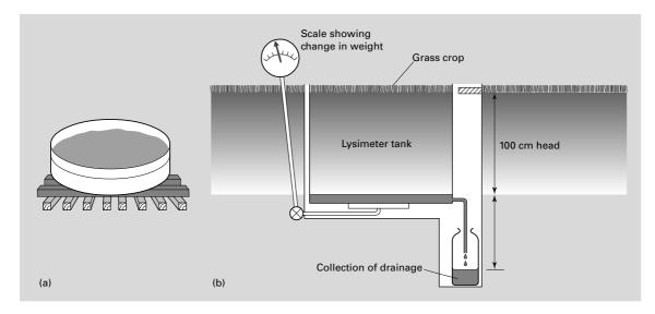
Fig. 6.15 (a) Class A evaporation pan. (b) A weighing lysimeter (after Pereira, 1973).
