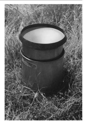
Fig. 6.3 A standard raingauge.
