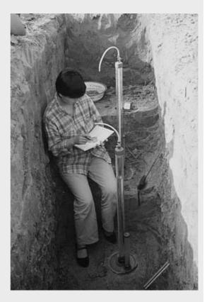
**Fig. B6.6.1** Disc permeameters in use for hydraulic conductivity measurements on a deep loamy soil on the North China Plain.
