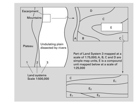
Fig. 14.6 'Nested' arrangement of soil mapping units.
