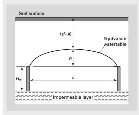
Fig. B13.7.1 Diagram for Hooghoudt's 'equivalent flow' model to drains (after Smedema and Rycroft, 1983).
