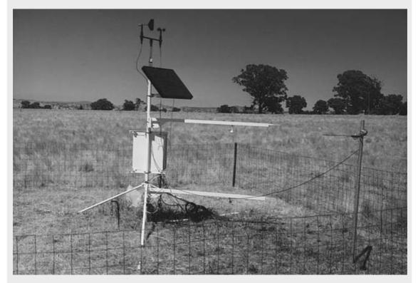
Fig. B6.9.1 A field installation for measuring weather and other variables for Et and the Bowen Ratio.
