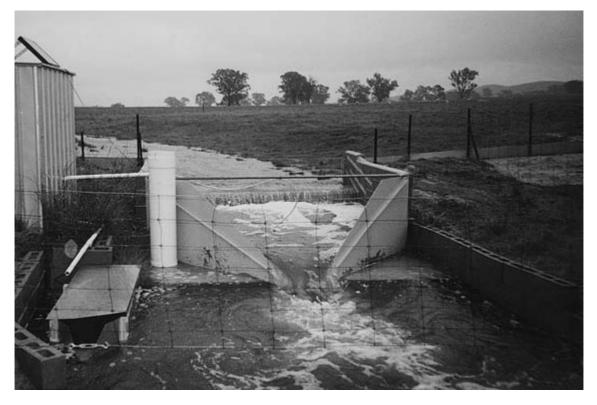
Fig. 6.4 Surface runoff being measured in an H-flume.
