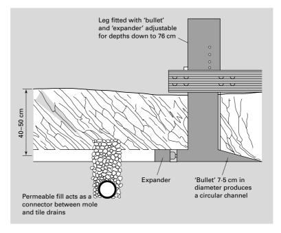
**Fig. 13.13** Diagram of a mole drain plough in operation (after MAFF, 1980).
