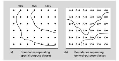
Fig. 14.4 (a) and (b) Soil boundaries drawn from grid surveys (after Beckett, 1976).
