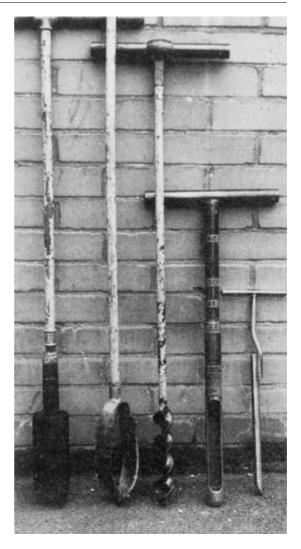
Fig. 14.1 A selection of augers and core samplers used in soil survey.
