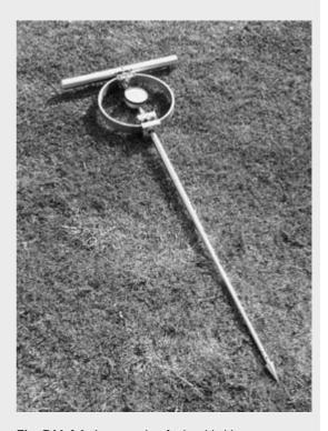
Fig. B11.6.1 An example of a hand-held penetrometer (after Davies et al., 1993).
