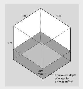
**Fig. B4.6.1** Diagram of a 1 m<sup>3</sup> soil cube filled with water to 250 mm depth (after White, 2003. From *Soils for Fine Wines* by Robert E. White, copyright © 2003 by Oxford University Press, Inc. Used by permission of Oxford University Press, Inc.).
