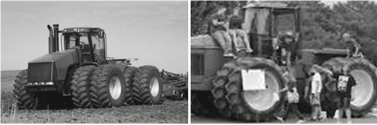
Fig. 2.2 Heavy farm machineries that can seriously compact soil
