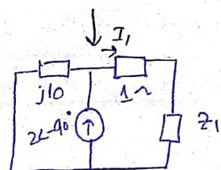
$$\text{So, } V_3 = I_1 R = \frac{j10}{(1+j10)+0.8-j1.6} (-j2) \times (1\Omega)$$
