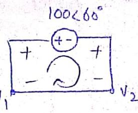
$$V_1 = V_2 + 100 \angle 60^\circ \quad (1)$$
