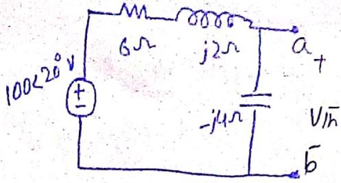
$$V_{Th} = 63.24 \angle -51.56^\circ \text{ V} \quad \text{Ans:-}$$
