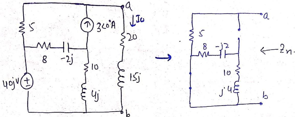
current passes through short-circuited easiest path through  $5\Omega$  so;  $Z_N = 5\Omega$
