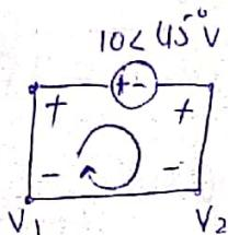
$$\rightarrow 3 = \frac{V_1}{-j3} + \frac{V_2}{j6} + \frac{V_2}{12}$$
