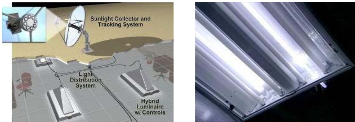
Figure 5-27. Hybrid Solar Lighting. Illustrations from Oak Ridge National Laboratory.
