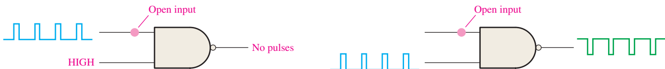
(a) Application of pulses to the open input will produce no pulses on the output.
