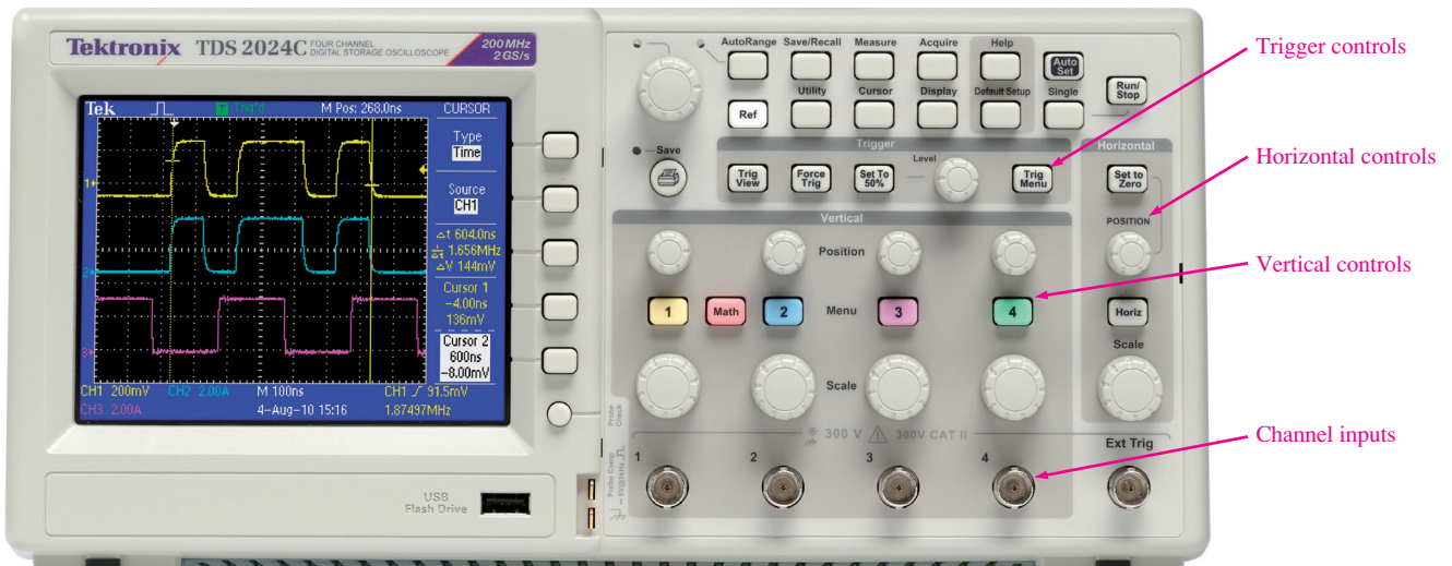
FIGURE 1–44 A typical digital oscilloscope front panel. Numbers below screen indicate the values for each division on the vertical (voltage) and horizontal (time) scales and can be varied using the vertical and horizontal controls on the scope. Used with permission from Tektronix, Inc.
