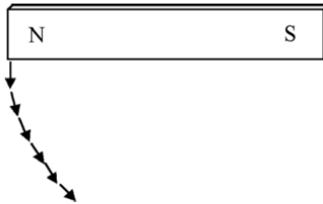
Figure 3.3: Constructing Magnetic Field Lines
