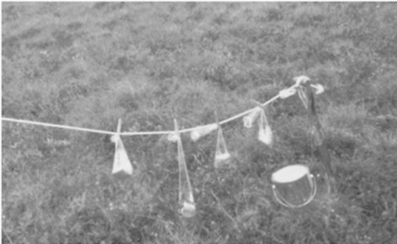
FIGURE 7.7 The cold method is a useful technique to determine soil bulk density under field conditions. The
