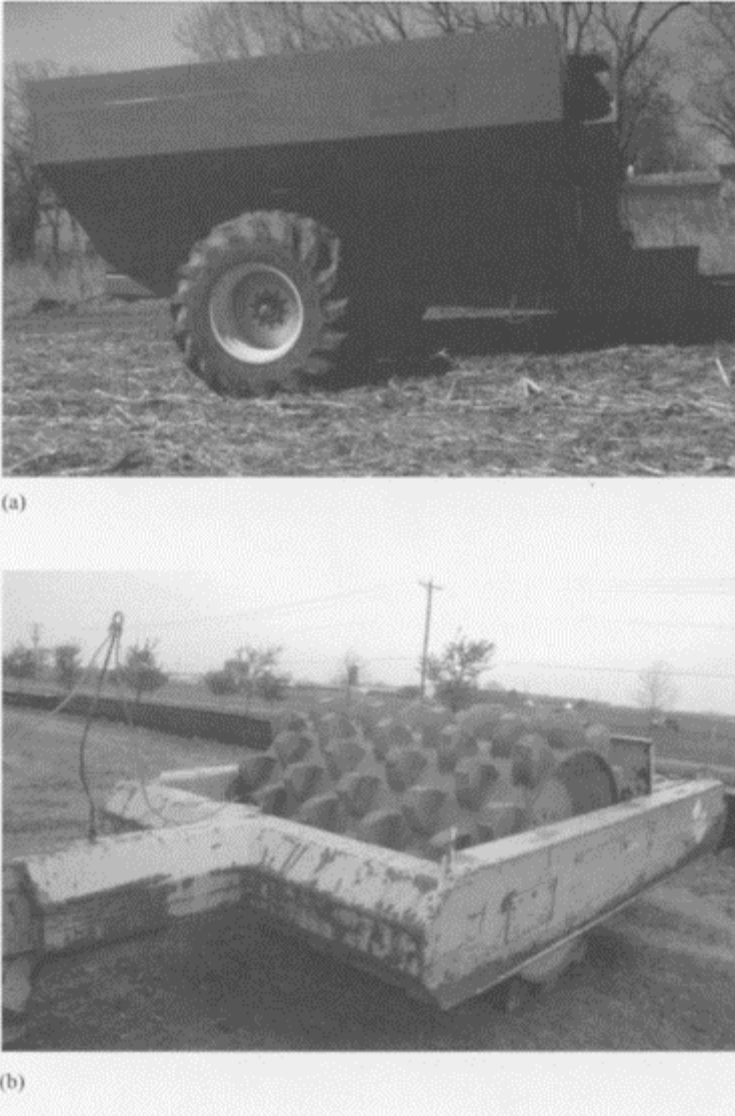
FIGURE 7.5 (a) A single-axle grain cart with capacity of 10 or 20 Mg can cause severe compaction during harvest in the fall, (b) A kneading roller is used to create a compact road bed. Spikes cause more compaction than a smooth roller.
