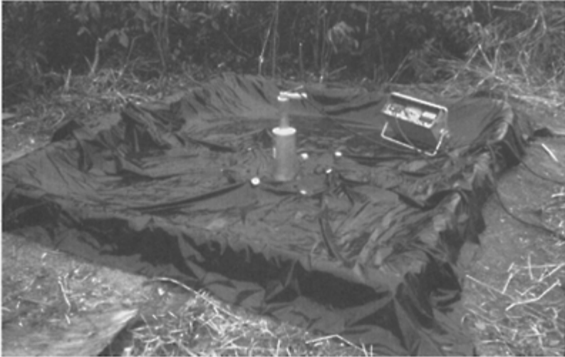
FIGURE 10.9 A plastic covered plot is used to assess field water capacity using a neutron moisture meter. After saturating the plot with sufficient water, the plastic cover was used to prevent evaporation. (Ibadan, Nigeria, 1971)
