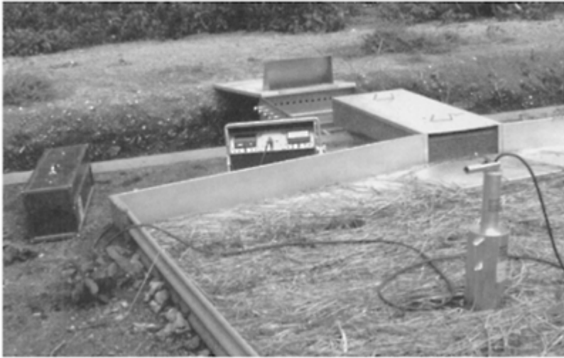
FIGURE 10.8 A neutron moisture meter with sealer/rate meter device. Some models have a rate meter built within one assembly (Ibadan, Nigeria, 1972).
