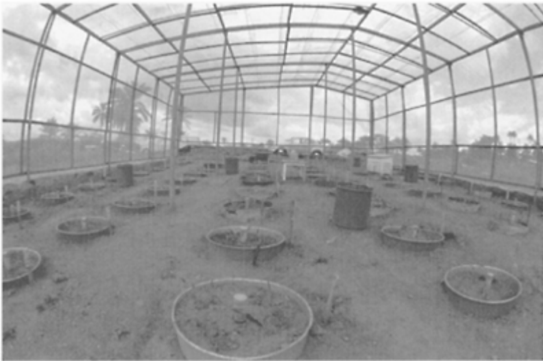
FIGURE 9.25 A series of lysimeters under a plastic shelter.
