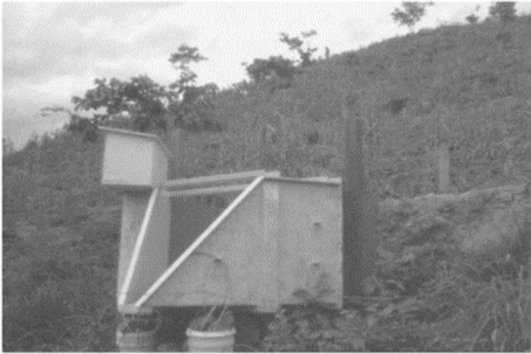
FIGURE 9.16 An H-flume and a water stage recorder to measure runoff from a steep agricultural watershed.
