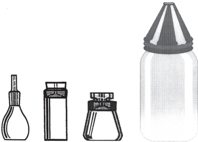
Fig. 2.2-1. Stoppered bottles used in the pycnometer method to determine particle density.
