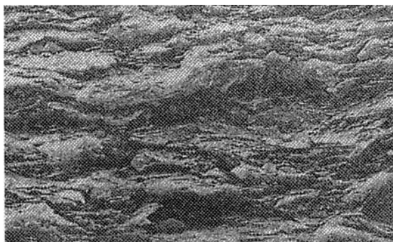
Fig. 6.13 Fissile shale viewed with an electron microscope ( \times 1000 ).
