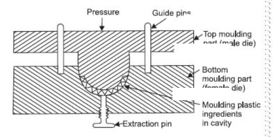
The raw material on becoming soft due to heat forces into air areas of the cavity because of applied pressure. The temperature and the pressure are continued to be applied till the chemical changes have taken place. The two parts of the die ore then separated and the molded article is taken out for cooling.
