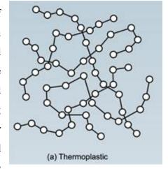
granular or fibrous materials. Thermoplastics comprised of Acrylic, Poly vinyl chloride (PVC), Poly ethylene, Poly vinyl acetate, Cellulose acetate, Poly propylene etc.
