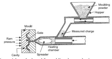
the mould and the process repeated. It is a quick method used for molding thermoplastics.
