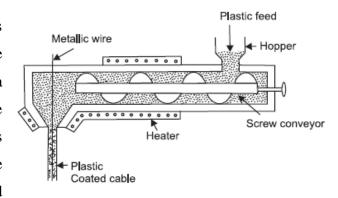
tubes are extruded through dies. If, however, something is to be provided with the plastic covering like insulation of electric wires and cables then the same is drawn through a die.
