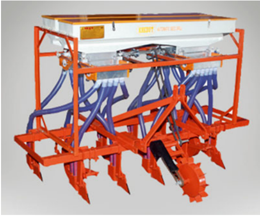
Fig. 13.3 Photograph showing zero-tillage sowing implement
