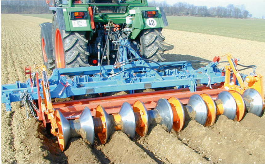
Fig. 13.4 Ridge-till farming system
