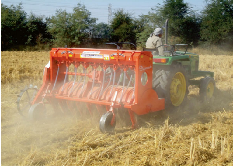
Fig. 12.4 Happy seeder for sowing in presence of residues (Photo courtesy: CSISA (CIMMYT-IRRI), New Delhi)
