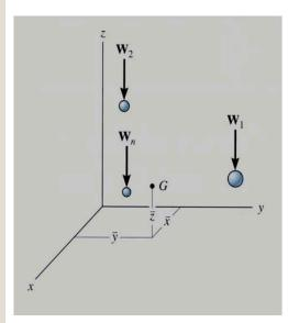
Consider a system of *n* particles as shown in the figure. The net or the resultant weight is given as  $W_R = \sum W$ .
