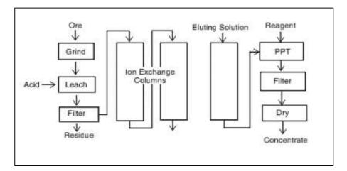
• Uranium is absorbed on the anion exchanger in fixed ion exchange columns. The absorbed uranium is passed by strong sodium chloride solution through saturated resin column:
