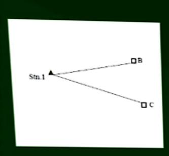
An angle is define as a different in direction between two convergent lines.
