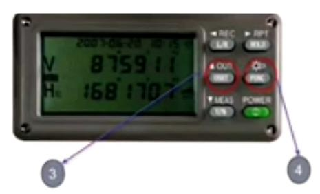
Export key: Press it under shift mode export current angle to serial port and to record with electronic controller
