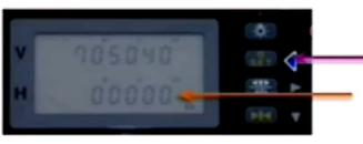
Horizontal angle is set to zero in A direction
